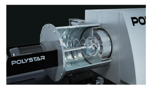
Automatic pelletizing speed adjustment - Produces more uniform-sized pellets without labor intervention
