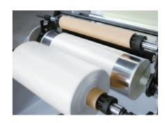
The twin head blown film machine allows producers to make different sizes of film width on the same machine on each winder at the same time (simultaneously).
